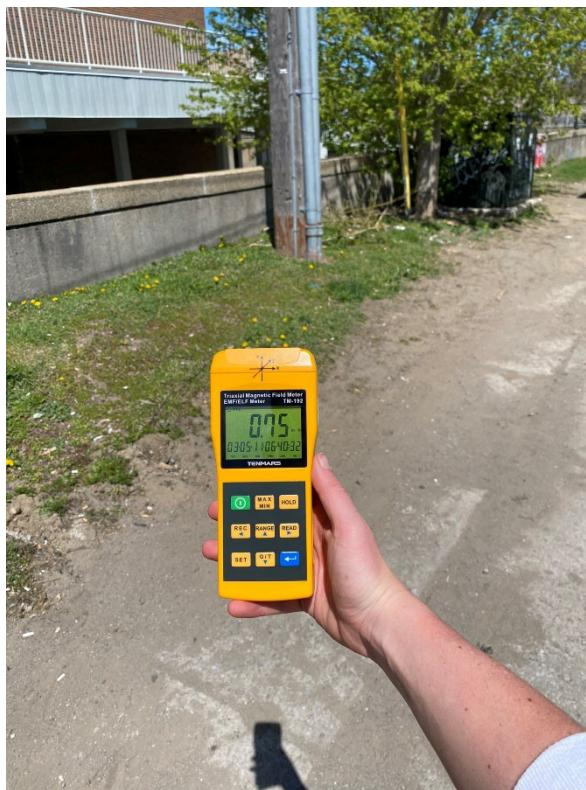
Figure 6: Elevated A.C. magnetic field readings recorded near existing Toronto distribution lines.
